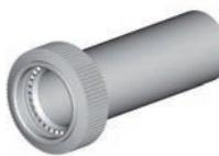
**Type 4:** Backshell derived from Type 3 without the cable gland. Suitable to adapt specific male threaded adaptors (not supplied) for ANAMET or PMA tubes for example. See table p.40 for the size of the female thread depending on the shell size.
