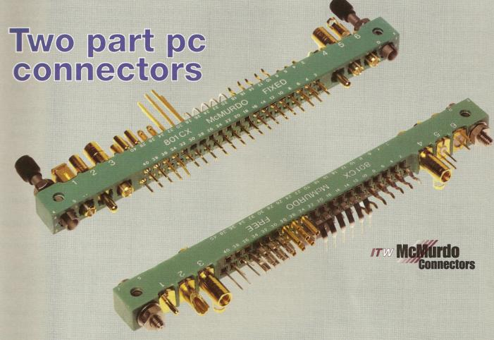
The 801 and 801CX Series two part printed circuit board connector system utilising a 1.27mm (0.05in.) staggered pitch with 2.54mm (0.1in.) between rows has been designed to satisfy the latest requirements of various UK and international standards including BS9525 F0006, BS9525 F0012, BS9525 F0027, BS9525 F0041, NFC 93-424 (HE 801 and HE 807), MIL-C-55302 and approved to BS9525 N0001.
